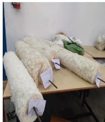
Figure 2. Blended Fiber rolled on the rod
